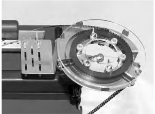
*Looper 8 is fixed with two M3 screws onto the bracket with the holes looking upwards. The position of the Looper 8 in the axis of projection and rectangular to it is important. With the help of the elongated holes in the foot of the looper the horizontal position can be adjusted. The film must run down straight vertically into the projector.*
