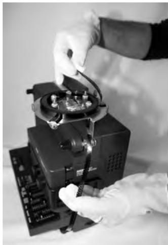
*The film roll is now placed on the Loofer 8. The cover made of acrylic glass must be removed and the perforation of the film must point **upwards**. It is important that the start of the film goes through the center hole of the looper ring. It must lie nicely around the needle bearings. The film is touching the looper only in three places, namely on the black plastic barrels which stand out slightly from below.*
