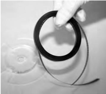
*The start of the film is hanging down on the inside now and the end of the film on the outside. It is ready to be placed on the looper.*
