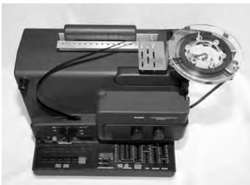
*If the buckle is significantly too long it can be shortened by opening the loop and winding the film end an additional time around the wound spool of film on the looper.*
